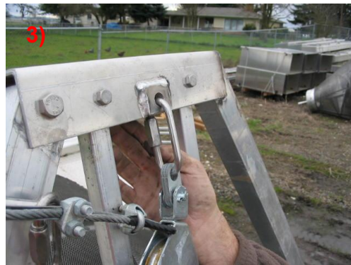
Stringing the cable for a 5-ft trap is illustrated in these pictures.
